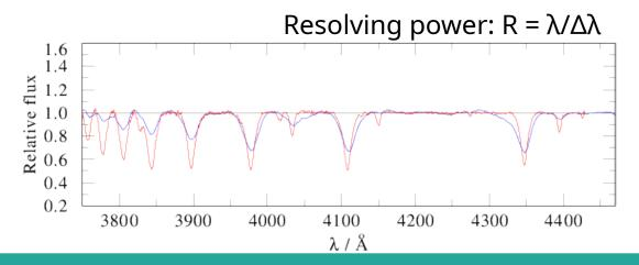
blue and red spectra were taken with the 200 lines/mm and 900 lines/mm gratings, respectively.
