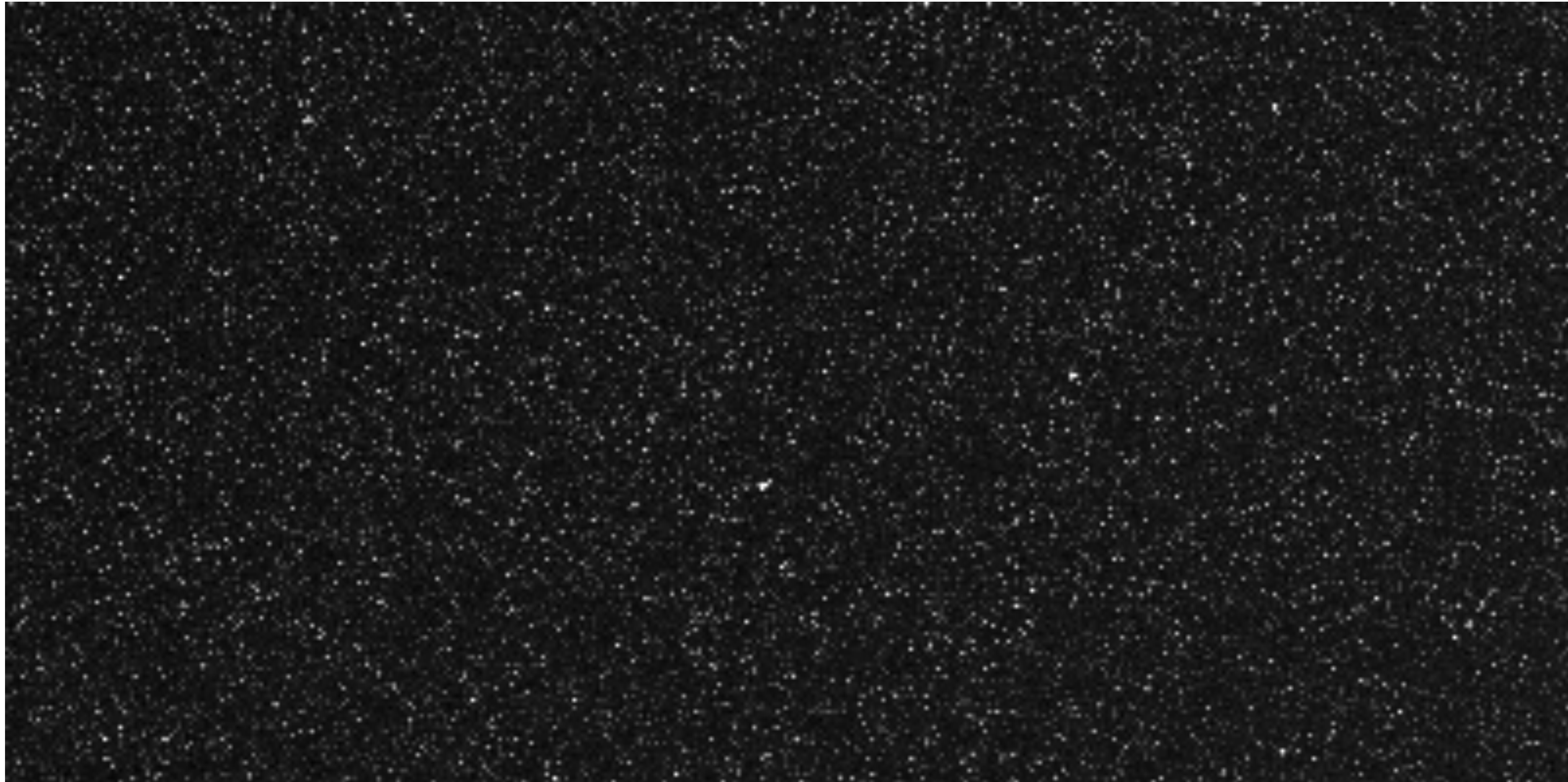
Figure: Dark frame detail: median of five 3600s exposures (log scale).
